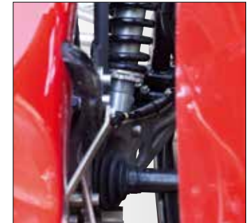
Chassis: Alloy semi-trailing link axle with adjustable Bilstein threaded suspension and 3 selectable springs: soft, medium, hard.
