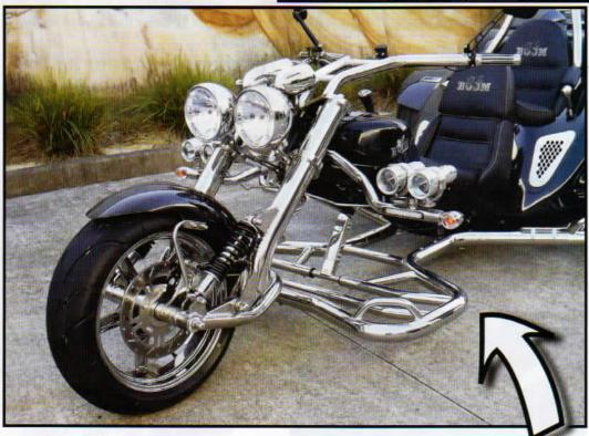
The Jet Light system accessory allows the spot lights to turn with the steering
