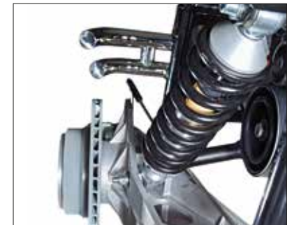
Chassis: Alloy semi-trailing link axle with adjustable Bilstein threaded suspension and 3 selectable springs: soft, medium, hard.
