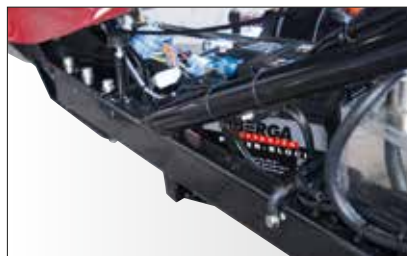
Frame: Plastic coated with car standards (salt spray test 600 h). Increased corrosion protection by 4-phases handling. Thick wall-thickness. Buckling resistant and optimal riding quality.
