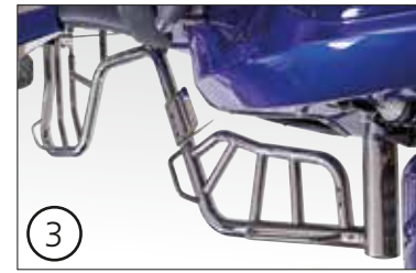
Leg protection bar and luggage rack, stainless steel, Ø 60 mm
