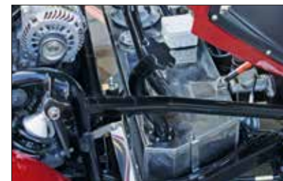
Attachment parts: Over 50 new stainless steel parts instead of galvanized or coated parts, as stainless steel tank, expansion tank, engine holder, gear box holder, engine facing, coolant facing, handbrake facing, air shields, miscellaneous small parts as well as all mounting parts.
