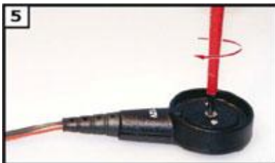
5. Close housing with screw - Ready!
